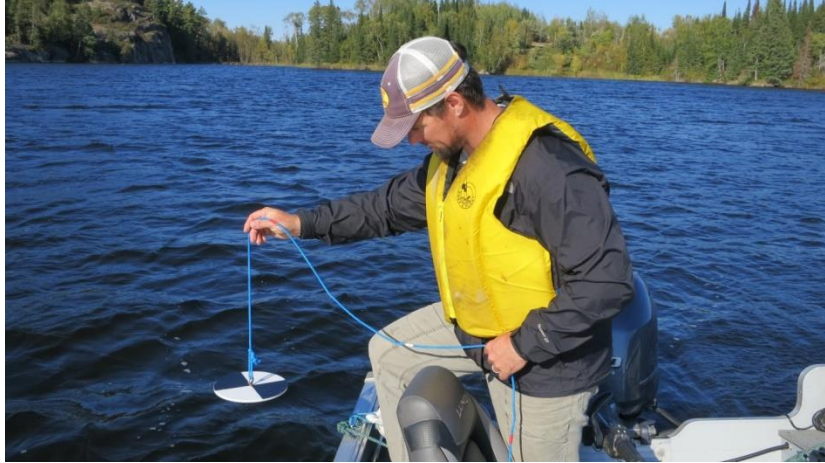
Figure 2 – Lowering of Secchi disk
