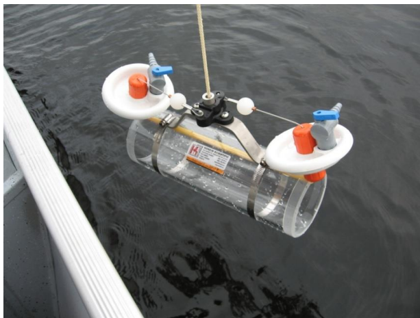
Figure 4 – Horizontal Beta Sampler prior to deployment
